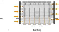
Rectangular paving stones can be shifted in a running bond by screwing pressure-rolls on the aligning bars.
