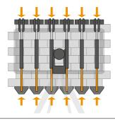
The 6 individual clamp arms are connected by spring steel strips to ensure the right pressure on each point of the layer.
