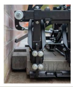
Paver layer sizes of 0.6 m<sup>2</sup> (6,5 ft<sup>2</sup>) to 1.5 m<sup>2</sup> (16 ft<sup>2</sup>) can be laid without problem
