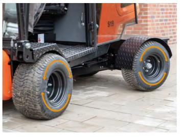
All 4 wheels are driven and braked hydrostatically.
